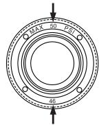
Air cap number located on face of cap. Cap number must correspond with baffle number to assure 10 PSI cap pressure.
