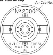
Maximum air pressure required to assure compliance of 10 PSI max. cap pressure - this reading must be taken at the spray gun handle inlet fitting.
