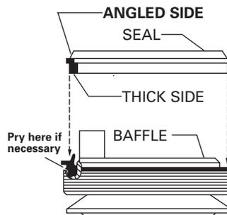
4. Assemble seal to baffle with angled side up as shown in diagram. **NOTE:** The seal should be a tight fit on the baffle. If it is a loose fit on the baffle, assure that it is assembled with the angled side up.
