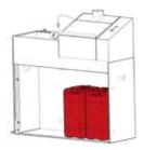
The drum to the left will contain the clean solvent. Connect the adapter plug with the single hose to it.
