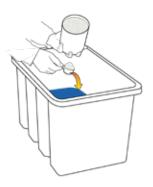
4. Pour the water into the filters to remove the paint from the water.
