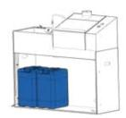
The drum to the left will contain the clean water. Connect the adapter plug with the single hose to it.
