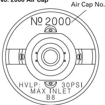
Maximum air pressure required to assure compliance of 10 PSI max. cap pressure – this reading must be taken at the spray gun handle inlet fitting.
