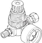
Use to maintain nearly constant outlet pressure despite changes in inlet pressure and downstream flow.
