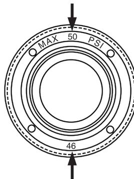
Air cap number located on face of cap. Cap number must correspond with baffle number to assure 10 PSI cap pressure.
