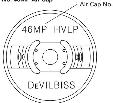
The 46MP Air Cap doesn't have markings showing the maximum air pressure required to assure compliance of 10 PSI max. cap pressure. That value is located on the front of the baffle. (See view below.)
