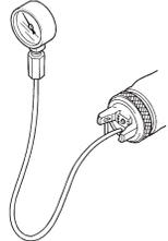
The purpose of this test kit is to measure air cap atomizing air pressure at the center air port of the air cap. Used to confirm code compliance and as a daily quality control measure.
