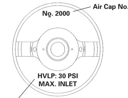
Maximum air pressure required to assure compliance of 10 PSI Max. Cap Pressure - this reading must be taken at the spray gun handle inlet fitting.
